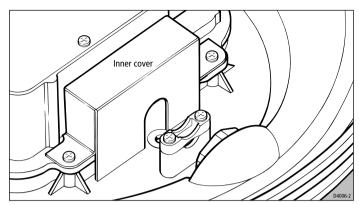
Remove the drain tube from inside the base of the scanner, and insert it into the drain hole as shown in the following diagram. Pull the tube gently from outside the scanner so that it clips into place.
